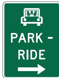
Typical MUTCD trailblazer sign for Park-Ride facilities
